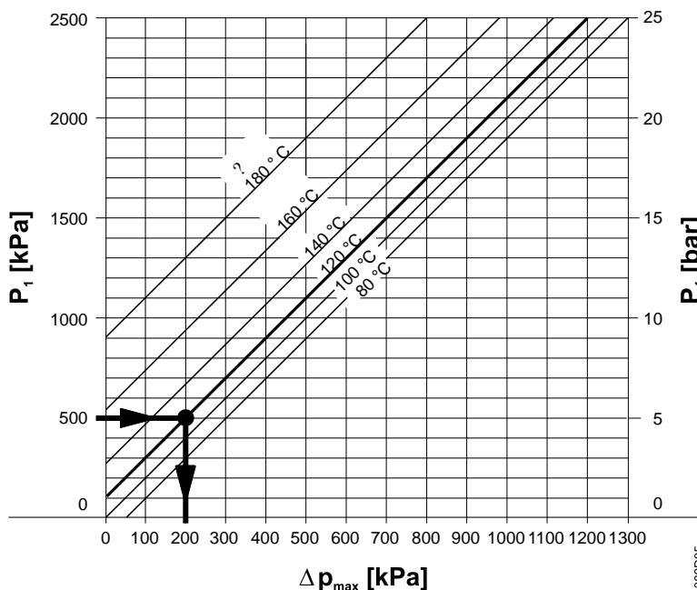
$\Delta p_{\max}$  = Differential pressure at a nearly closed ball valve to largely avoid cavitation
