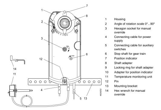
Arrangement for shaft adapters
