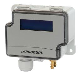
DPT-Ctrl differential pressure controllers are designed for building automation systems. Controller can control constant pressure or flow of fans, VAV systems or dampers. When controlling air flow, it is possible to select a fan manufacturer or a common measuring probe that has a K-value.
