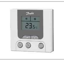
REPI series thermostats are used to control room temperature in industrial, commercial and residential environment via controlling electric modulating valve with 0-10VDC (4-20mA) control signal or floating control as well as damper actuator of VAV system.
