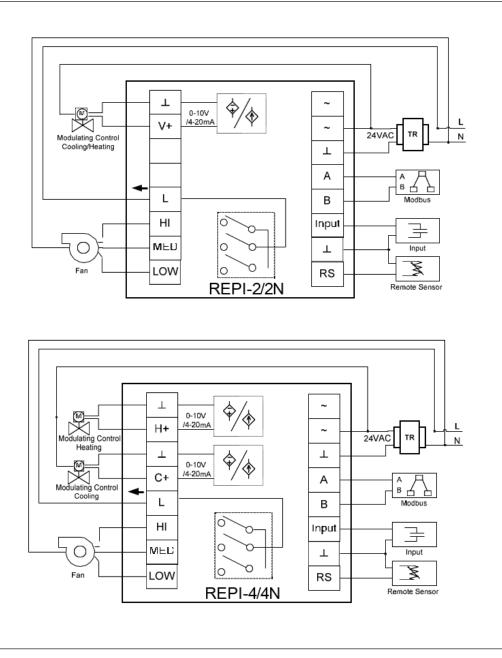
Note: Be sure to connect all the wires as per the wiring diagrams and keep it away from water, mud and other material so as to prevent the unit being spoiled!
